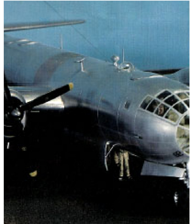
In this view, you will note that two figures have been added to the bomb bay area. Simulating armament specialists, these figures are ideal for camouflaging the electrical wires that lead to the lamp in the forward bomb bay.
