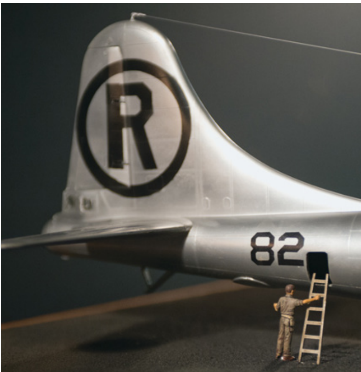
As you will quickly discover, the "Superfortress" model is extremely tailheavy and somewhat difficult to balance. Although a mounting screw was added to the nose gear assembly, it was decided to reinforce the entire model by opening the rear crew entry and positioning a boarding ladder in the doorway as shown.
