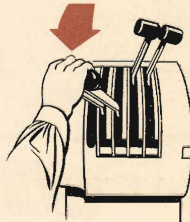
LOW BLOWER TO HIGH BLOWER
