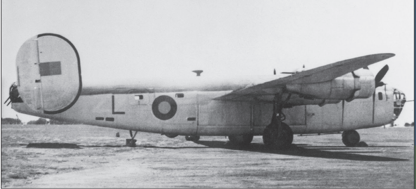
Liberator GR Mk.V BZ826 "L", No. 200 Squadron, St. Thomas Mount base, Madras, India 1944. In February 1944, the squadron was ordered to move from Africa to India. Majority of its aircraft reached the Indian base on the break of March and April. The plane already bears the ACSEA markings. Notice the Boulton-Paul Type E tail turret with black framing.
